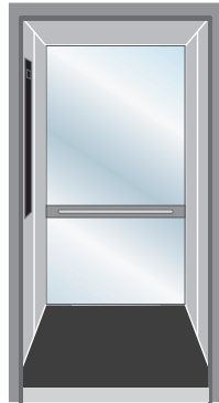
mirror VSG 6 mm crystal, glued on wall, with a handrail
