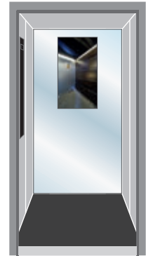
mirror VSG 6 mm crystal, total height, with a monitor behind the mirror
